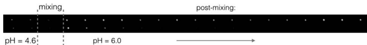
13 14 15 16 17 18 19 20 21 22 23 24 25 26 27 28 29 30 31 32 33 34 35 36 37 38 39 40 41 42 43 44 45 46 47 48 49 50 51 52 53 54 55 56 57 58 59 60 Figure 1: A montage of TIRF frames at 2 s per frame for two representative particles illustrating the main states along the experimental procedure: pre-mixing, transient defocusing due to mixing and equilibration, post-mixing. There is clear post-mixing intensity increase.
